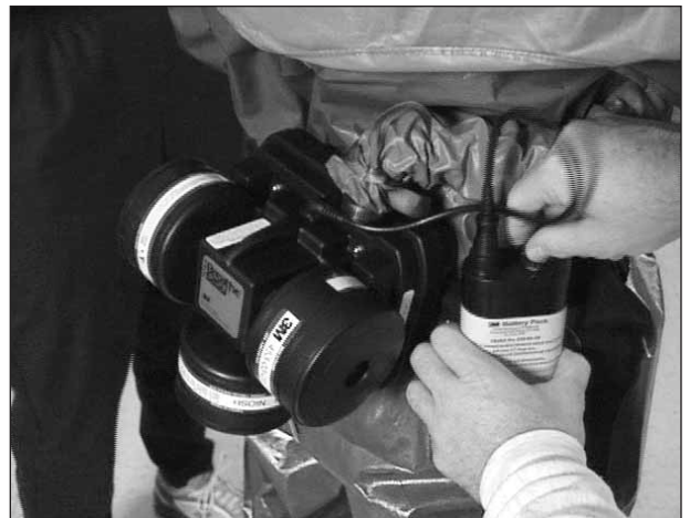
Connecting and inspecting the PAPR battery.
