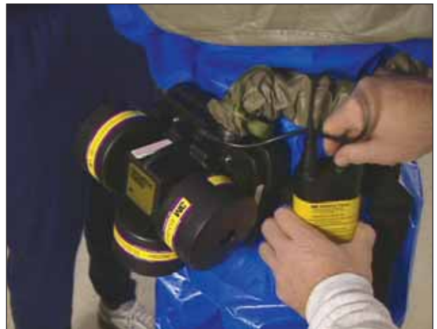
Connecting and inspecting the PAPR battery.
